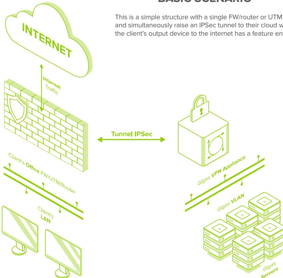
This is a simple structure with a single FW/router or UTM to get the client's traffic to the internet and simultaneously raise an IPSec tunnel to their cloud with Gigas. This model only requires that the client's output device to the internet has a feature enabling IPSec tunnels to be activated.
